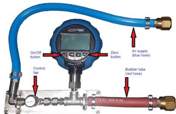
Bubbler setup with Additel gauge
