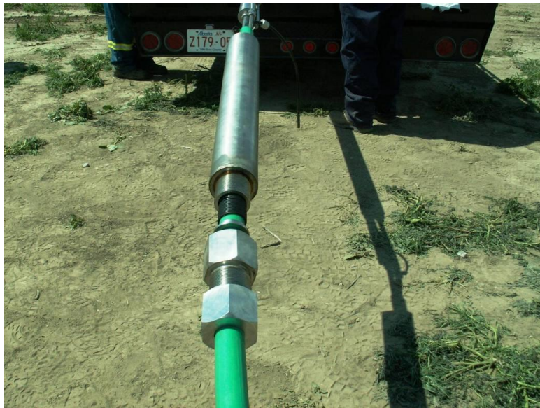
Pic 4. An Airwell Pump with Umbilical Coiled Tubing attached
