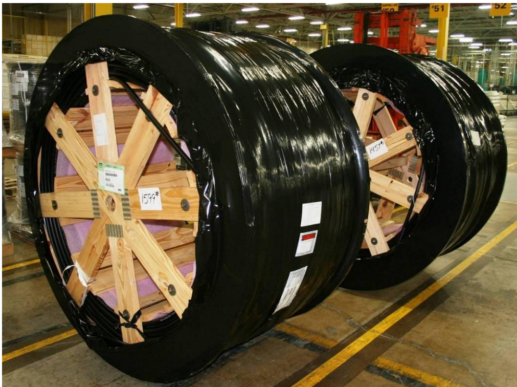
Pic. 8 Reels of High Pressure 1/2" Redistribution Line (approximately 11,500 feet)
