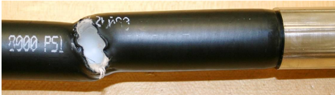
Pic. 7 Photo of initial "Burst Test"
