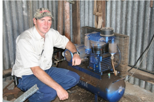
Off Peak Power: David Bunge with his Airwell compressor which powers his pumps on off peak electricity
