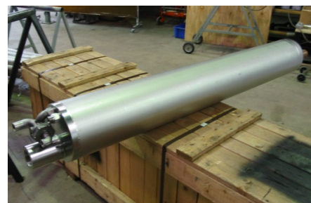
Custom made 8" by 1.6m Airwell pump for Tamala Park
