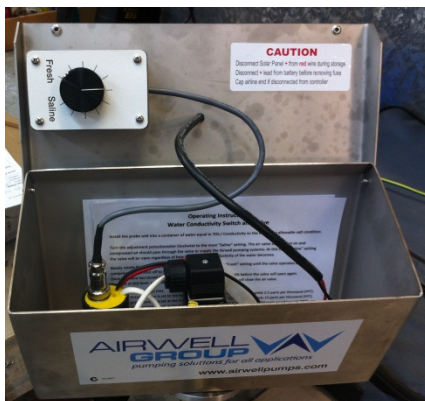
Airwell controller with inbuilt salinity sensor
