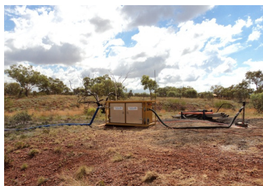
Airwell flow testing skid setup on one of the testing bores
